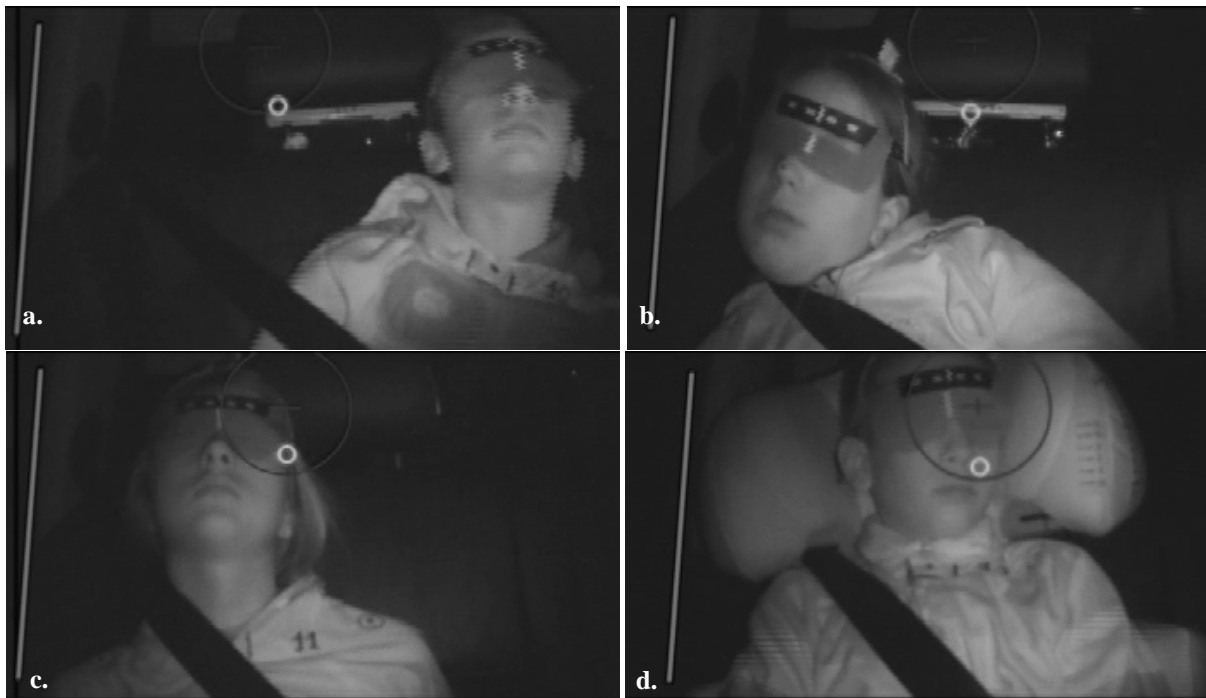
Figure A2: Illustrations of the various belt fit definitions. a) Off of the shoulder – the belt crosses the upper arm lateral to the acromion. b) Into neck – the belt is visibly pressing into or supporting the neck. c) Sternum – any portion of the belt crosses the occupant midline superior to the sternal notch marking. d) No “poor” belt position notes.
